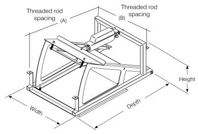
\* Mounting hole dimensions 6mm dia
